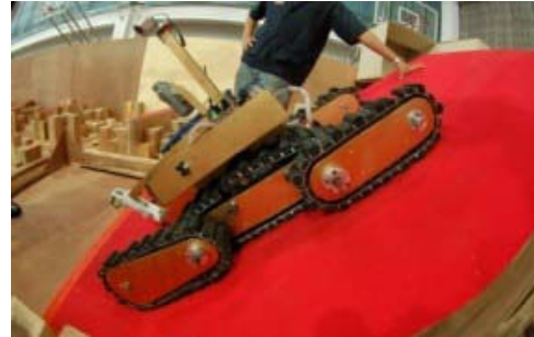
Fig. 3 The Tehzeeb is on a 45 degree testing slope
