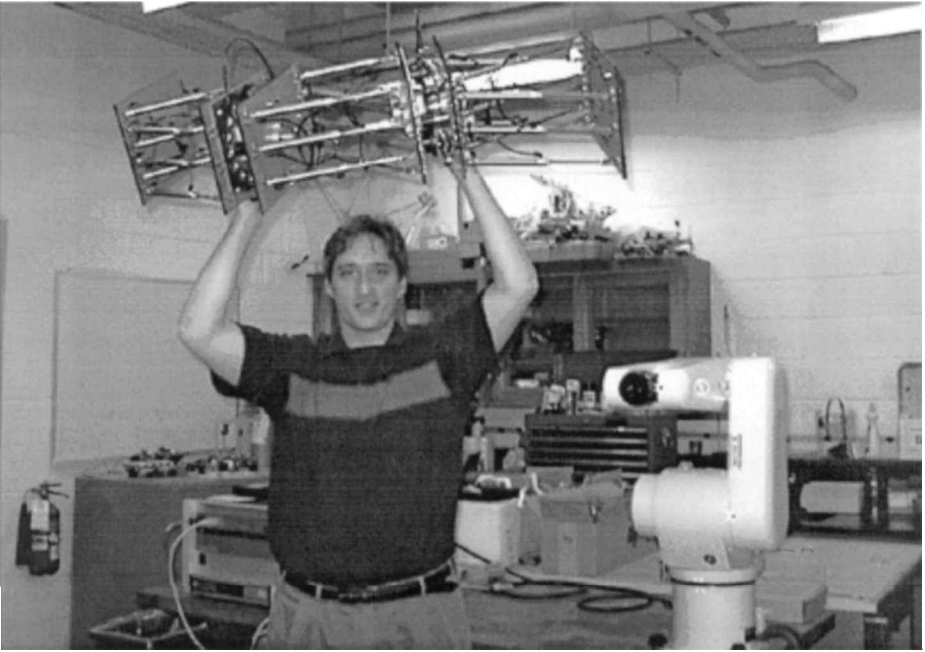
Figure 8. The light weight of the new manipulator is illustrated in comparison with traditional manipulators.
