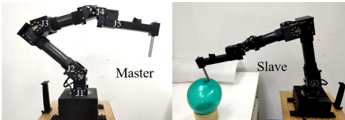
Figure 11. Bilaterally controlled 5-DOF manipulator
