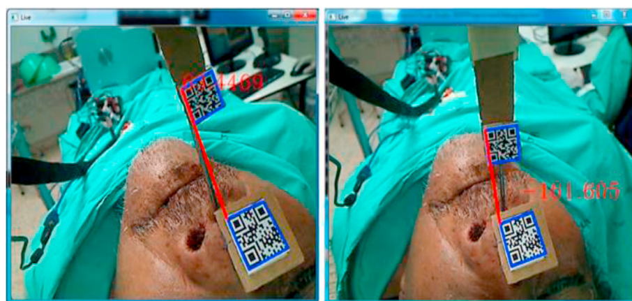
Fig. 6. QR code tracking system (Open Source Computer Vision Library) associated with the robot guiding EETS. QR code tracking from monitor display view.
