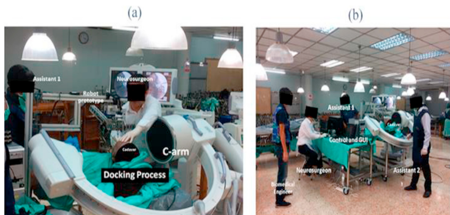
Fig. 7. The EETS experiment on cadaver. a) The prototype Robotic system assisting the neurosurgeon in the EET approach; b) The overview of the operating room with the position of the whole team consisting of neurosurgeon, assistant1, assistant 2, biomedical engineer and the orientation of the cadaver and robotic system during EETS robotic approach.
