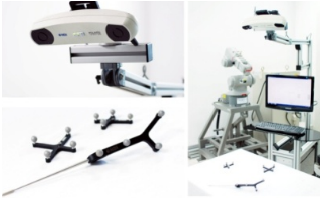
Figure 2. The Optical tracking system and the passive marker.
