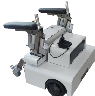
Fig. 1: Mobility assistance robot developed in BART LAB intended to assist sit-to-stand, stand-to-sit and walking
