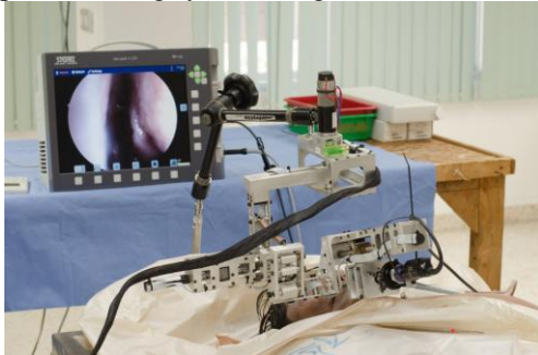
Fig. 1 BART LAB EETS robotic platform in cadaveric experiment.
