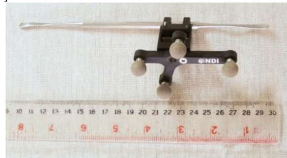
Fig. 2 Medical tool attached with optical marker.
