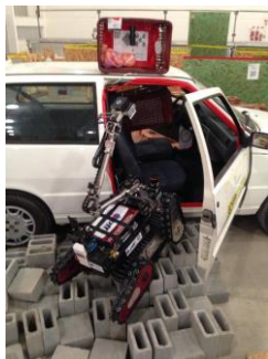
Figure 3. Extended manipulator of Tele-Op IV reaching the victim at red zone in World RoboCup 2014, Brazil.
