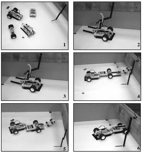
Figure 7: The Self-Replicating Process of the Robot 3.
