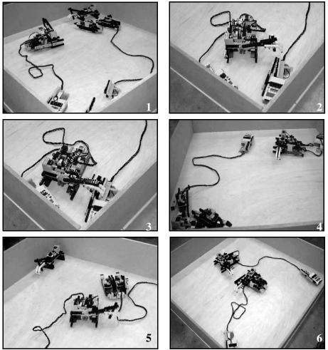
Figure 9: The Self-Replicating Process of the Robot 4.
