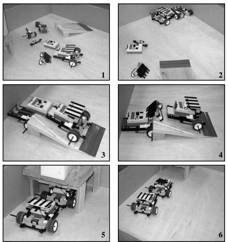
Figure 3: The Self-Replicating Process of the Robot 1.
