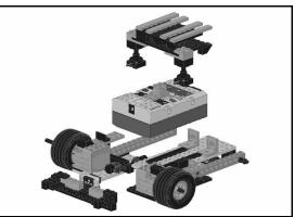
Figure 2: The Exploded View of the Robot 1.
