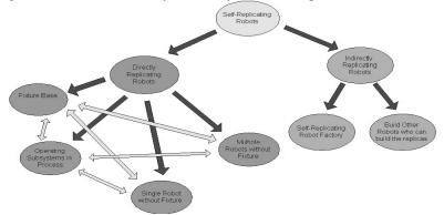
Figure 1: The Block diagram of the categorization of self-replicating robots.
