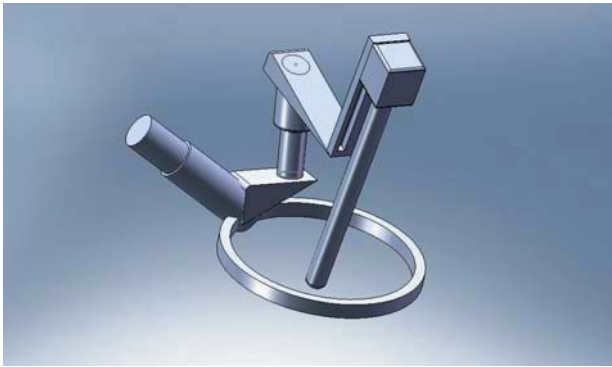
Figure 8. Structure of the new laparoscope-holder robot.
