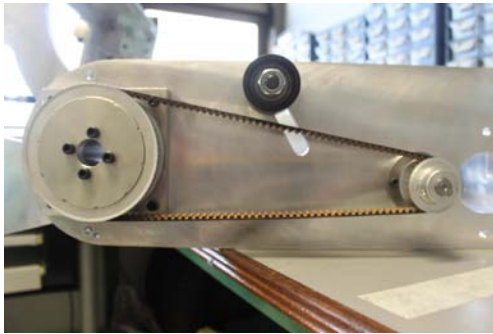
Figure 13 Driven mechanism of circular motion
