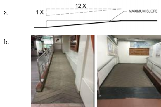
Figure 1. The slope example in hospital standard environments and real hospital environment a) standard slope in hospital building standard guild [10] b) slope in rural hospital environments.
