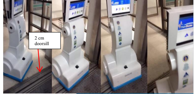
Figure 12. Experiment moving through doorsill high 2 cm in tele-operation mode.
