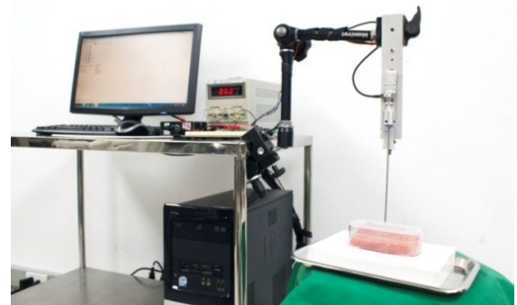
Fig. 3. Experiment set up with the needle insertion robotics system with F/T sensor, veress needle and a control computer for the data acquisition
