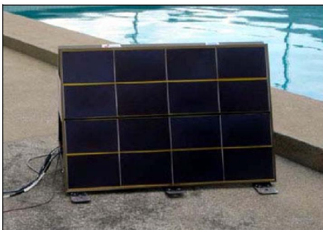
Fig. 12. Solar-Panel System (On-Site Robot Battery Charger)
