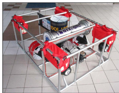
Fig. 17. The final version of the ThaiXPole underwater robot
