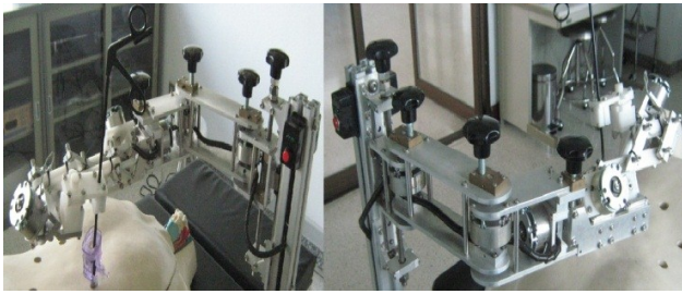
Fig. 1: Passive MU-LapaRobot (Passive Surgical Tool Holder).
