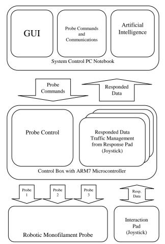
Figure. 4. Schematic control of the diagnosis system includes; system control PC, control box, robotic monofilament probe and interaction pad.
