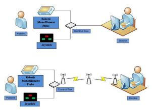
Figure. 3. System diagram: GUI and Controller Command, Control box, and Robotic Monofilament Probe.
