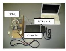
Figure.9. System of the prototype "Robotic Monofilament Probe"
