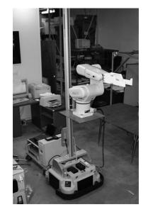
Figure 1: The vertical translation system integrated with the robot manipulator.
