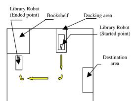
Figure 7 (a): Robot motion planning of the path section 1.
