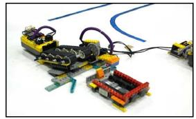
Figure 5: Activation of station 1 when the chassis triggers the station's light sensor.
