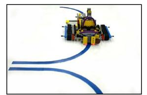
Figure 3: Robot1 autonomously tracking a painted line with the light sensors.
