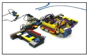
Figure 7: Activation of station 2 when the chassis triggers the station's light sensor.
