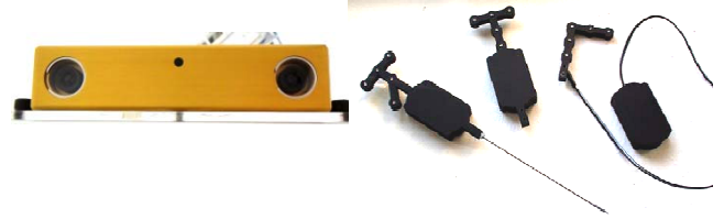
Figure 5. (a) a Bumblebee stereo camera. (b) an optical marker in different pattern.
