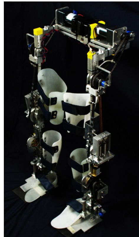
Figure 14. The new motorized-mechanical exoskeleton
