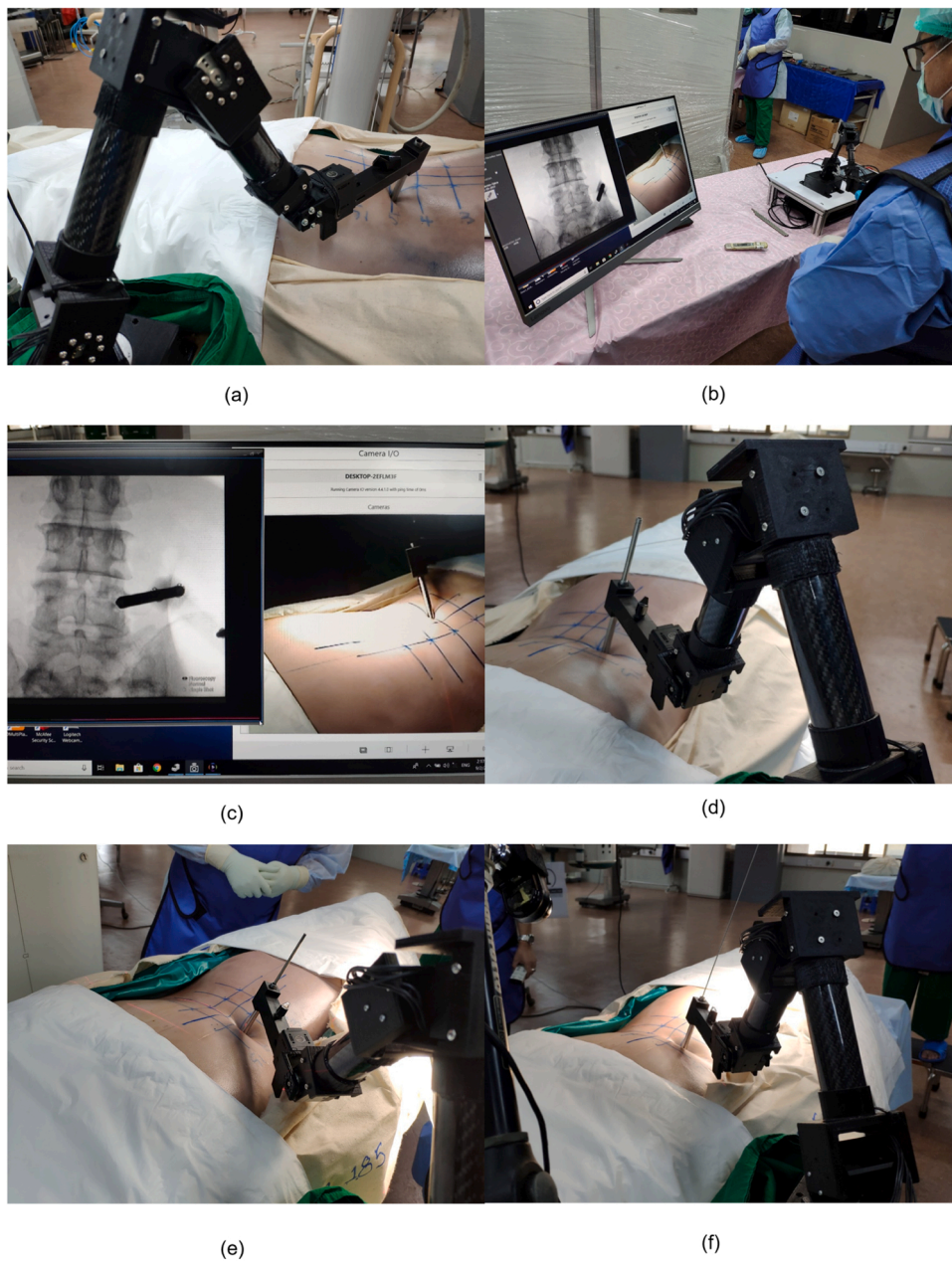
Fig. 8. Robot-assisted pedicle screw Insertion (a) The slave manipulator placed to the entry point of pedicle (b) Surgeon controlled the master manipulator at workstation (c) The real-time fluoroscopic x-ray and patient video image. (d) The small, guided sleeve inserted into end-effector of manipulator (e) The percutaneous pin traversed a guided sleeve and penetrated the pedicle (f) The K-wire inserted into the pedicle.
