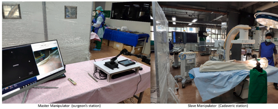
Fig. 7. The robot assisted percutaneous pedicle screw insertion: experiment setup.
